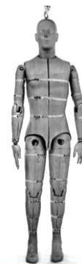
"Sierra Sam," developed for the U.S. Air Force in 1949 to test ejection seats, represented the median height and weight of the 50th percentile adult male U.S. population.
